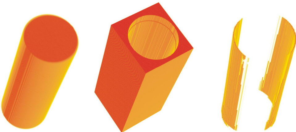
Figure 7. Combination of cylinder (left) and borehole (middle) variant volumes to generate a statistical collision region (right)
