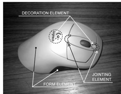
Figure 2 Form elements of a mouse
