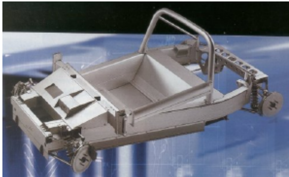
Figure 1. Lotus Elise aluminium chassis
