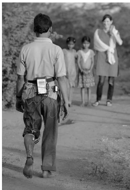
Figure 1. Biomechanical assessment of, in this example, barefoot walking on a natural substrate. Note the hip-mounted datalogger
