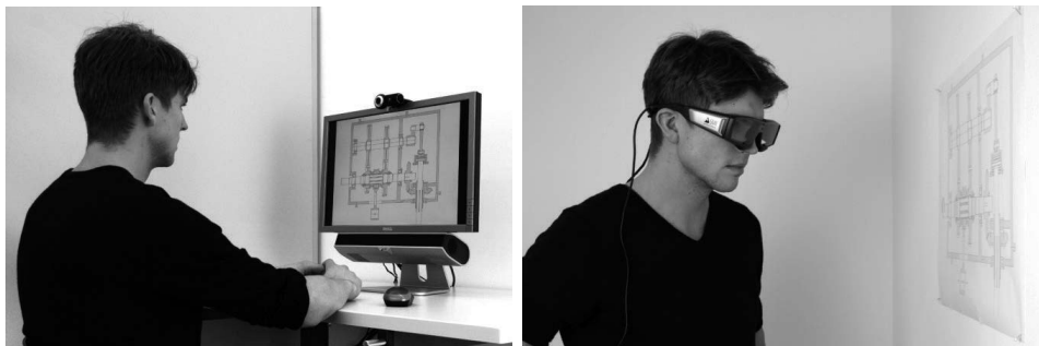
Figure 1. Eye tracking by a remote system (left) and by head mounted glasses (right)
