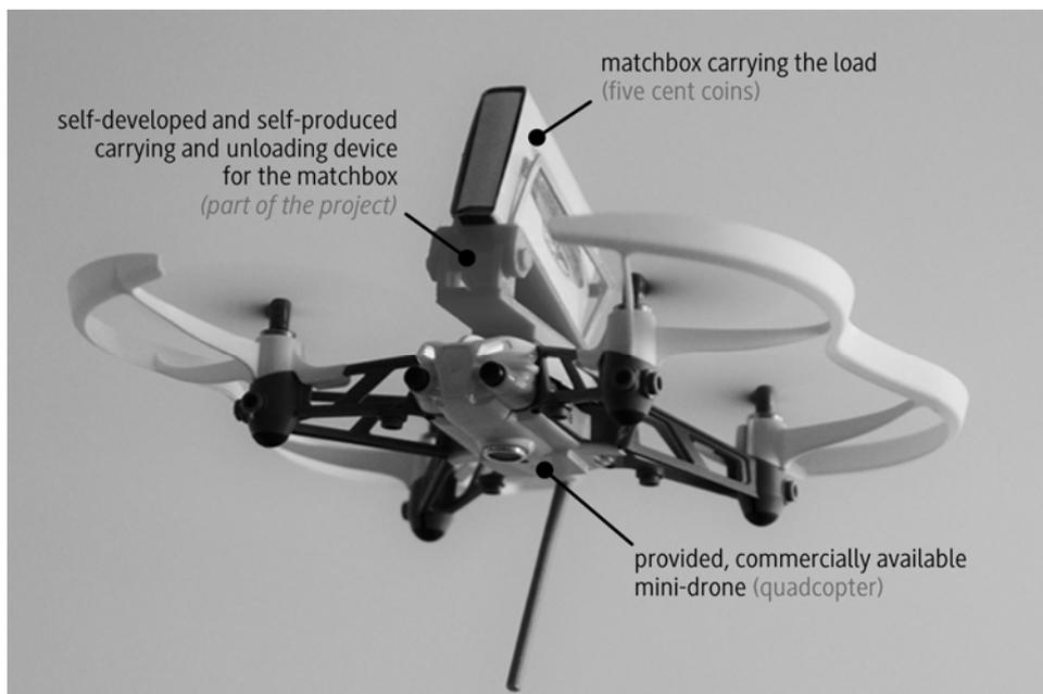
Figure 1. Assembled student-made device
